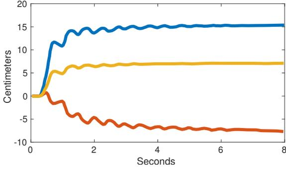
Fig. 5. Open-loop arm experiment, starting from a straight, down-hanging arm pose going towards a deformed state through an open-loop step actuation. The graph shows the x (red), y (blue) and z (yellow) positions of the arm's end-effector as it is swinging back and fourth while asymptotically nearing a straight arm pose.
